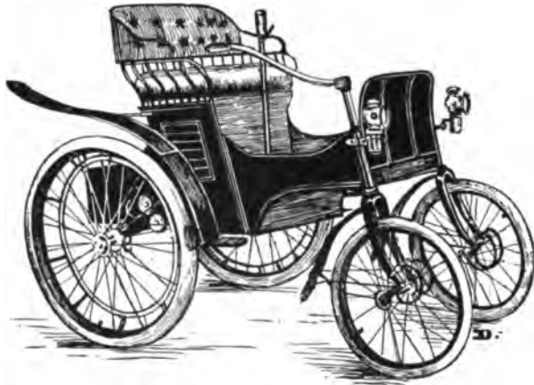
FIG. 22.—The Oakman-Hertel Gasoline Carriage, showing the steer wheels set in and turned by bicycle forks.
